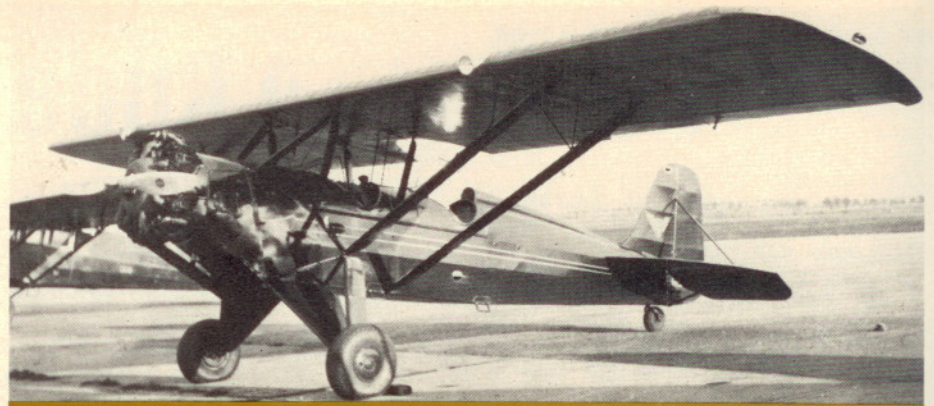
The prototype Timm Collegiate after extensive modifications that included new high vertical tail, modified turtledeck, redesigned landing gear, and a MacClatchie Panther engine. Fred Bamberger photo
