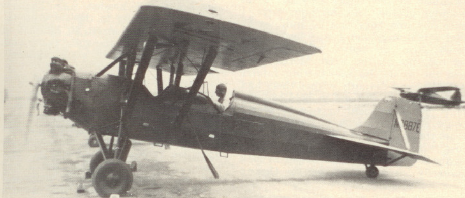
The second Collegiate , with tail revised to what could be called standard configuration (compare with No. 1), revised landing gear, and its fourth engine model, a 170 h.p. Curtiss Challenger.
